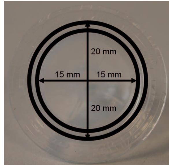
Figure 2: Dimensions of the simulated annulus.
