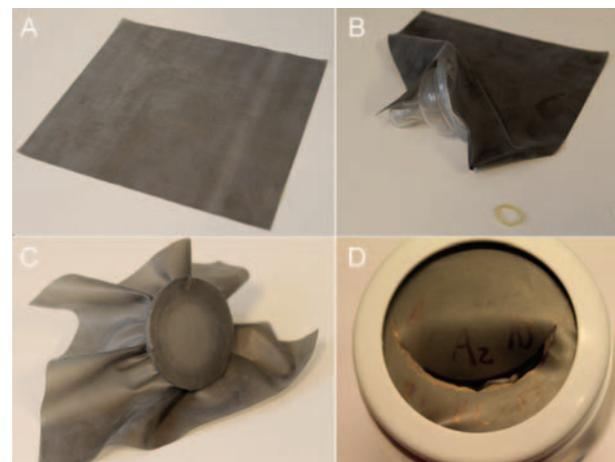
Figure 4: (A) Square sheet of dental dam. (B) Main simulation components; Feeding teat, dental dam, Tru-Force® elastic. (C) Assembled components. (D) Simulated leaflets and orifice.
