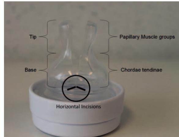
Figure 3: The subvalvular apparatus with simulated chordae tendinae and papillary muscle groups.
